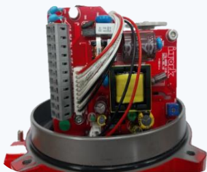
PCB with terminal blocks. Torque limiting by PCB (Option : Modulating type - Sending signal to PLC and make the motor stop running)
